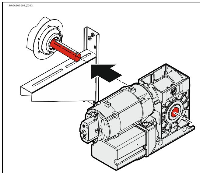
Tighten all connection elements (M12) to 75
