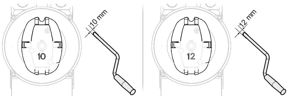
Plug in the crank and turn until it engages (①). Open or close by turning the crank (②).
