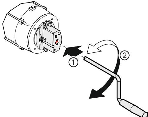
After use, the crank may be attached to the drive unit.
